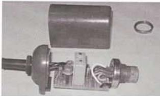
Figure 2. The stripboard and components with pressel switch casing
